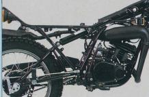
**Exclusive Monoshock rear suspension** allows greater rear wheel travel. This long stroke helps keep the rear wheel on the ground for better control, more comfort, and consistent traction on road or off.
