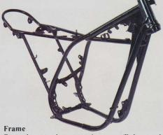
Over the roughest terrain, an off-the-road bike experiences punishment that would literally destroy even the best road machine, and at YAMAHA in order to assure dependability regardless of the condition of the trail or the amount of vibration generated by the spirited engine, a high-tensile-strength, double-cradle frame is utilized. This double-cradle design has become famous throughout the world for its ability to withstand the gruelling treatment of hill-climbing, jumping and motocross sports.
