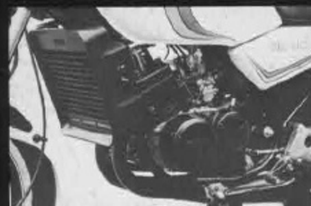
The compact power-unit. The aluminum corrugated pressure-type radiator has a sub-tank on the right side of the chassis.
