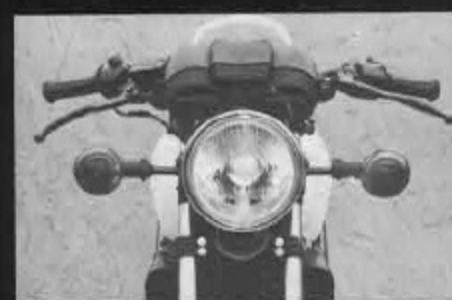
The 12V 60/55W halogen headlight. Radiator arrangement is also perfect.
