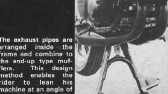
The exhaust pipes are arranged inside the frame and combine to the end-up type mufflers. This design method enables the rider to lean his machine at an angle of up to 55° on either side.
