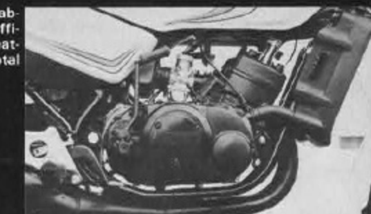
The exhaust pipes are arranged inside the frame and combine to the end-up type mufflers. This design method enables the rider to lean his machine at an angle of up to 55° on either side.
