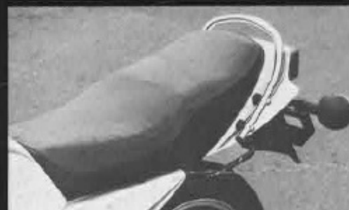
The newly designed seat. Small items are kept in a seat compartment or tail cowl.
