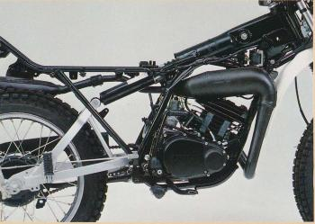
(Chassis: 2) The longer travel and the slower action of the monoshock suspension allow the rear wheel to follow surface irregularities, rather than bouncing over them. The ride is easier, progress faster, and maximum power is delivered to the ground. The rigid sub-frame keeps the wheel in alignment, minimizes weaving, and assists positive steering in the rough and on the road.
