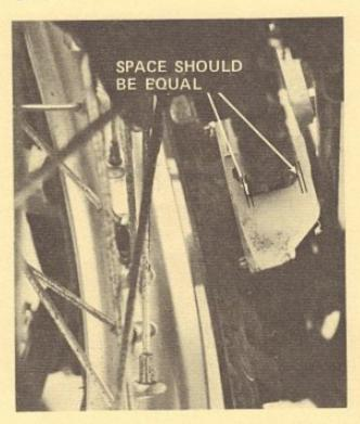
Instruct your customers to inspect the chain guide after each race. Rocks or other debris can bend the chain guide.
