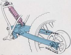
The DT125LC follows motocross practice with its rising-rate Monocross suspension allowing 210mm of wheel travel. The box-section swinging arm is controlled by a single gas/oil shock absorber (adjustable for spring pre-load) and rising-rate linkages that exert more pressure as the spring is compressed.
