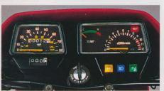
Even the meters in the instrument panel are thinner, to reduce weight at the steering head, The waterproof console contains speedometer, tachometer, temperature gauge and warning lights.
