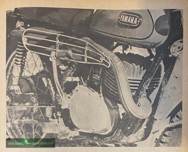
Simple 250 cc two-stroke single puts out 21 bhp and more than enough torque to push the machine through the most impossible country.
