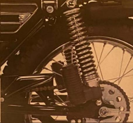
**Thermal-Phase rear shocks have built-in oil coolers to prevent overheating, no matter how hard or long you ride.**
