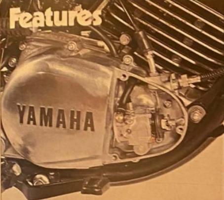
**Autolube**, a feature on most Yamaha two-stroke engines, automatically injects oil into the fuel mixture, so there's no need for pre-mixing. And, since it adjusts the flow of oil to engine load and speed, it extends engine life.
