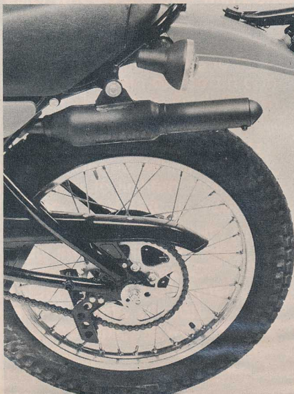
The swing-arm member rising from the axle adds to rear-end rigidity. Spark arrestor/muffler is effective.
