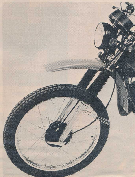
The center-axle fork with stylish dust covers allows seven inches of travel and has acceptable damping.
