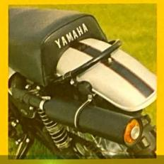
Super Silencer sifts the sound through a pulsating diaphragm, throwing the sound waves out of phase, and then, by means of an acoustic balance process, cancels out much of it.
