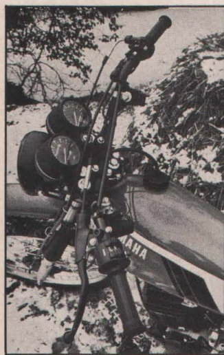
Unlike Suzuki, both Yam and Kawa had rubber sheathed levers but Yam 'bars and controls were overall tops (padding is missing from 'bars).
