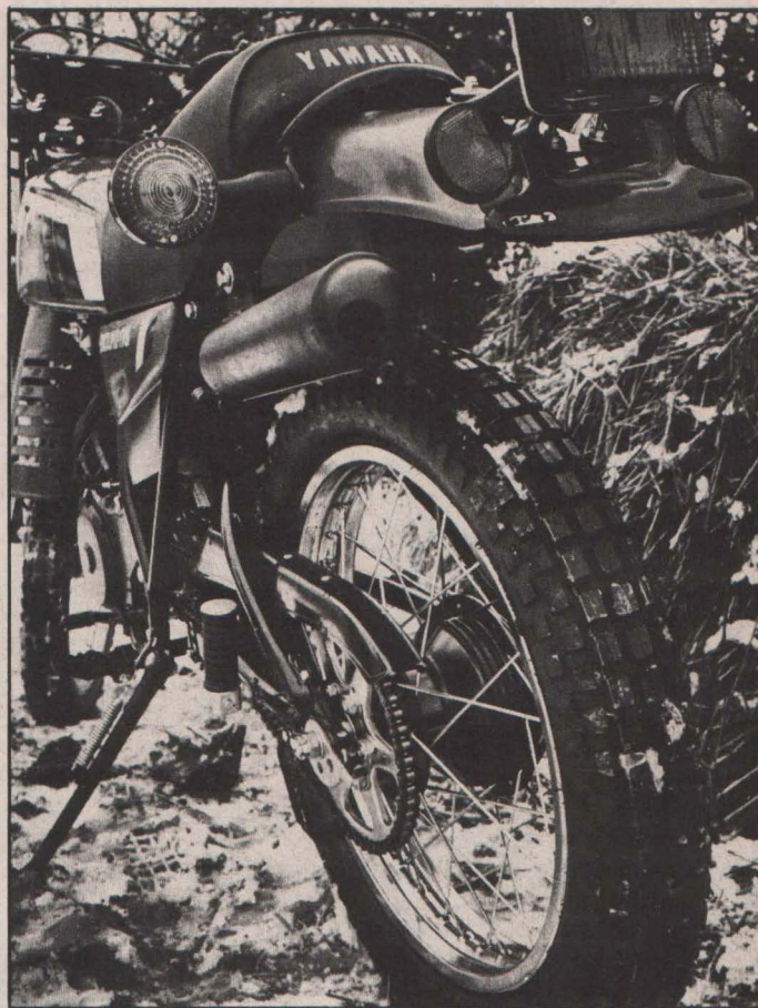
(Top left) Yam engine starts easy, pulls well. Note serrated fender, designed to pour mud all over fins! Slim Suzy tank needs key to fill 'er up (above left). DT's cantilever rear-end and snail cam adjusters are the bizniz (above right).
