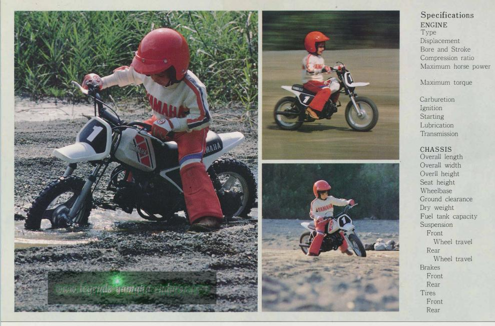
2-stroke single 49cm<sup>3</sup> 40×39.2mm 6.0:1 2.7hp(2.0kw) @5,500rpm 0.39kg-m(3.8 Nm) @4,500rpm Mikuni VW12 C.D.I. Kick Autolube Automatic Shaft drive 1.245mm
