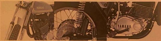
New high-clearance fender of lightweight polypropylene is virtually unbreakable. New front fork design and new steering geometry help 1974 Yamaha Trails handle like motocrossers on rough trails
